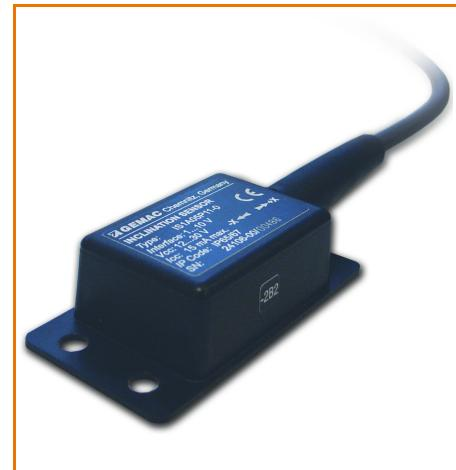
The inclination sensor IS1A xx Pyy / IS2A xx Pyy is available with a current loop or voltage interface. It enables the two-channel measurement of inclinations in the angle range (xx) of  $\pm 10^\circ$ ,  $\pm 45^\circ$  or  $\pm 60^\circ$  and  $\pm 90^\circ$ . The full-scale readings are calibrated factory-made at  $25^\circ\text{C}$ .
